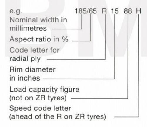
The speed code letter indicates the maximum permissible speed at which the tyre is to be operated.
