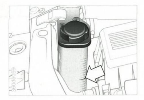
The picture shows (as an example) the coolant level equalising reservoir on cars with a spark-ignition engine. For the coolant level equalising reservoir on diesel-engined cars, see illustrations of engine compartment, starting on page 150.
