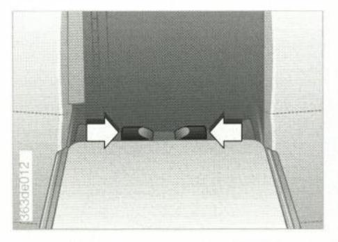
Remove the centre armrest. To do this, press the two levers together (arrows) and take the armrest out forwards.
