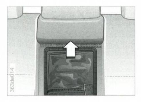
Press the knob (arrow) under the seat back fabric: this will release the flap in the load area, which will drop to the floor.
