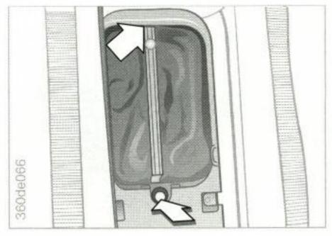
Press the circular button: this will release the loading flap in the luggage compartment.
