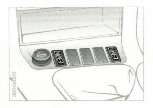
The seat cushion and seat back can be heated when the ignition key is in position 2.
