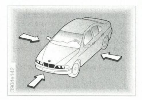
The picture shows the directions of impact to which the airbags respond in the event of a collision. Side protection is only available if the car is equipped with side airbags.
