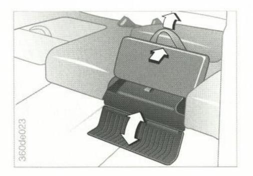
To obtain the desired "low" (stage 1) or "high" (stage 2) child's seat position, pull the loop strap and press the lower part of the child's seat down to the rear as necessary. After this, push the child's seat lightly forwards in the opposite direction so that it engages in the required position. Swing the footrest down.
