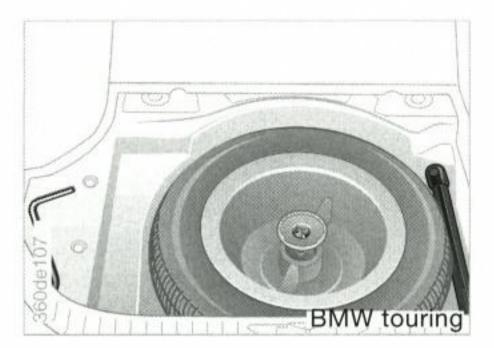
To avoid rattling noises later, make a note of how the various tools are attached to the car and replace them in precisely the same positions afterwards.
