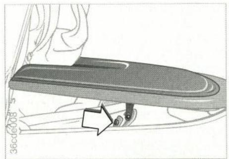
Unlock the soft-top compartment cover with the handle in the left rear side panel.
