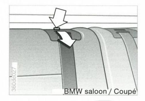
The rear seat back is split centrally. Either side can be folded down separately to accommodate lengthy objects.
