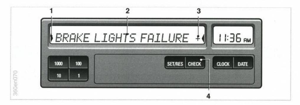
Faulty systems are shown by cleartext information or warnings. In addition, there is a warning light on the instrument panel.
