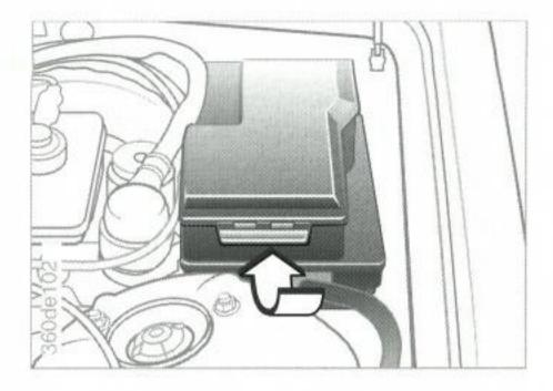
If an electrical consumer fails, switch it off and check its fuse.
