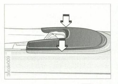
Close the soft-top compartment cover securely by pushing it down at both sides until it is heard to lock into place.
