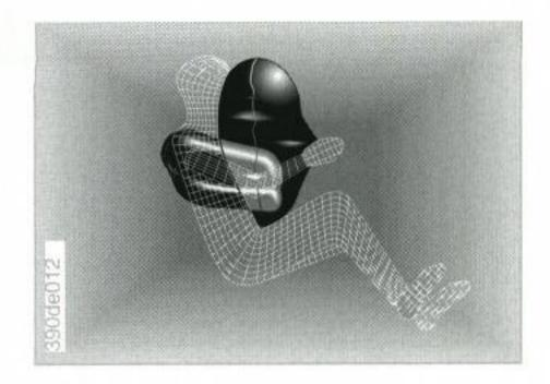
Retardation sensors continuously monitor the acceleration forces acting on the car. If a frontal impact causes the rate of retardation to reach a level at which the seat belts alone would not provide sufficient occupant protection, the gas generators for the driver's and front passenger's airbags are also ignited. However, the passenger's side airbag is not inflated unless a further sensor detects that the front passenger seat is occupied.
