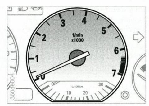
Never allow the engine to run in the red zone of the revolution counter.
