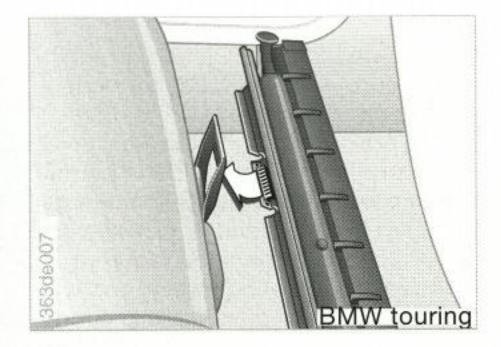
Before attaching the load-area net casing, make sure that the mountings in the rear-seat footwell and the catches on the casing are aligned.
