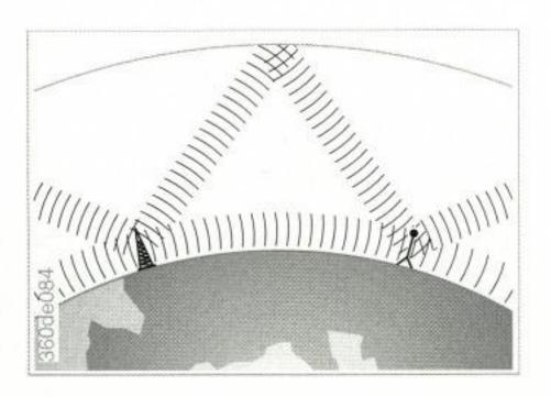
The longest reception range is obtained in the MW, LW and SW bands, since the signals are transmitted both as ground waves round the earth's surfaces and also reflected back to earth from the ionosphere layer in space.
