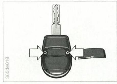
3 Remove the two screws (arrows) and take off the cover.
