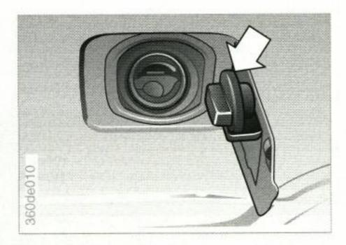
Releasing the fuel filler flap if the central locking has failed: see page 187.
