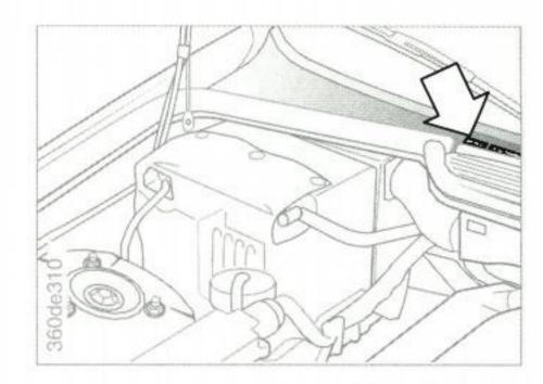
In the engine compartment, at the right on the heater bulkhead (arrow).
