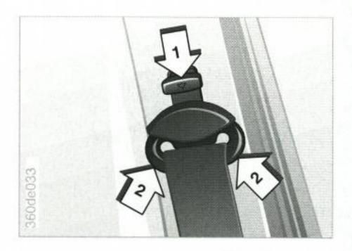
The seat belt height adjusters enable the belt run to be matched to the wearer's stature:
