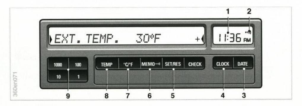
System malfunctions are shown in clear text by means of Check Control messages and warnings. There is also a general warning light on the instrument panel. For further details and operating instructions, see pages 76, 77.
