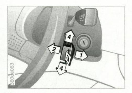
Any desired road speed above approx. 40 km/h (approx. 25 mile/h) can be memorised and maintained automatically.
