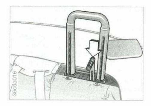
It is possible to retract the automatic roll-over protection system if it has extended unexpectedly.
