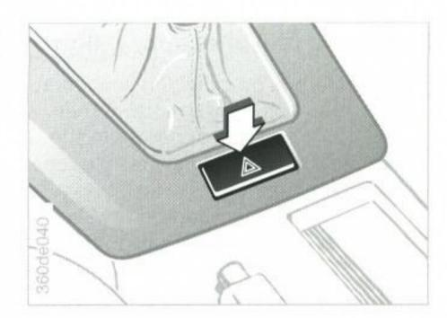
The pushbutton lights up in a regular rhythm when the hazard warning flashers are operating.
