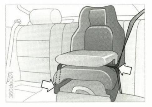
To install the extra-comfort seat back\*, place the head section over the head restraint.
