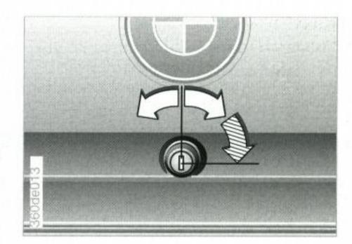
The lock can only be opened and closed with a master key.
