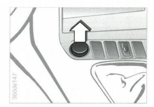
Remove the protective cap. The socket can be used for a 12 Volt hand lamp, car vacuum cleaner or similar appliance rated at up to approx. 200 Watts.
