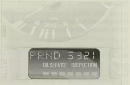
Your BMW's automatic transmission is equipped with Adaptive Transmission Control (ATC). This special feature selects from among a range of shift programs to precisely tailor the transmission's response to your individual driving style and requirements (including a special winter mode).
